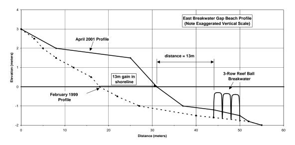
Figure 4. Beach Profile across Breakwater near East Gap
