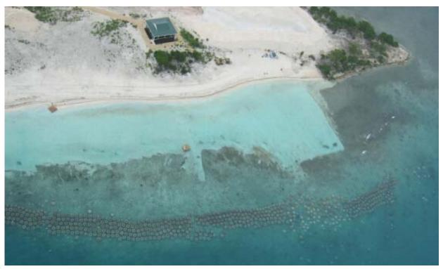
**Figure 8.** Aerial Photograph of 5-Row Reef Ball Breakwater in Antigua (Note that the breakwater also incorporates snorkel trails, swimming and diving areas.)
