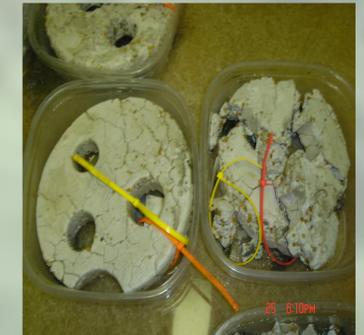
Figure 10: Discs made from 100% PoP (right) vs. an 80/10/10 mixture of plaster/sand/portland (left). Discs shown are approximately one month old.
