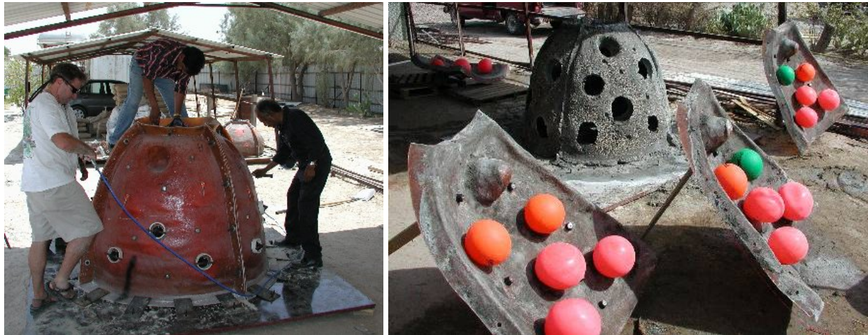
Figure 2. Traditional Reef Ball Unit Mold Fabrication
